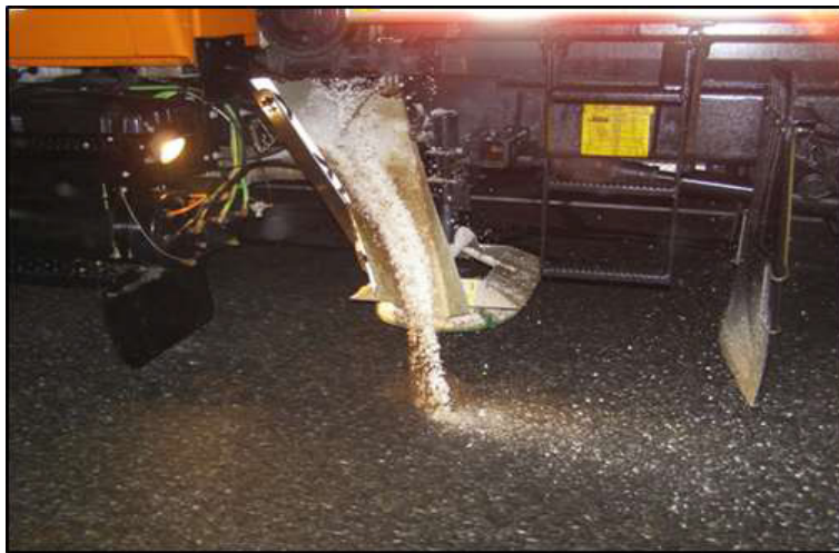
Figure 7: Salt, Pre-Wetted as Dispensed, Using a Static Spinner to Create a Windrow Application
