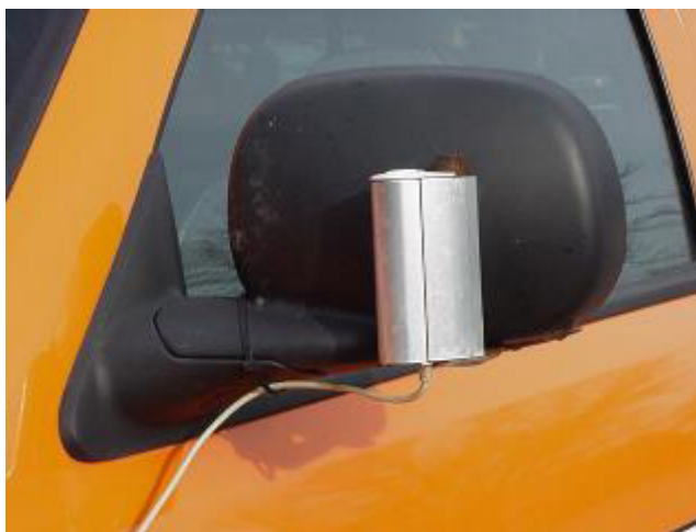
FIGURE 7.3. AIR AND PAVEMENT TEMPERATURE SENSOR (COURTESY IOWA DOT)
