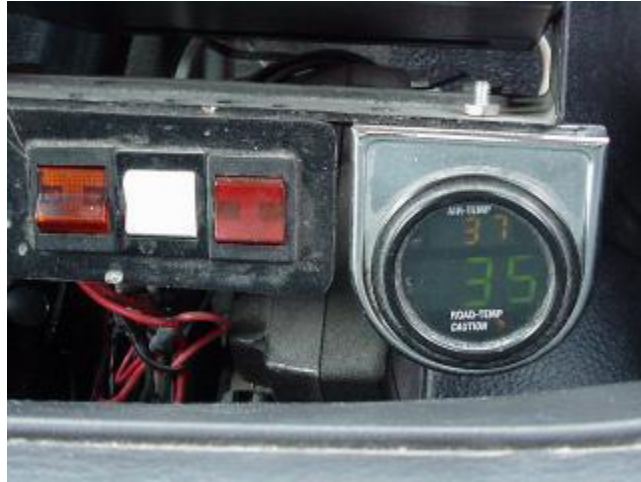
FIGURE 7.4. AIR AND PAVEMENT TEMPERATURE SENSOR DISPLAY (COURTESY IOWA DOT)
