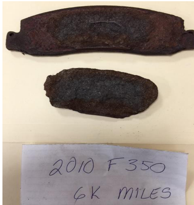
FIGURE 6.10. CORRODED BRAKE COMPONENTS (PHOTO FROM [126])
