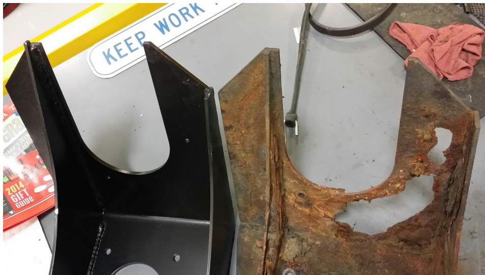
FIGURE 6.11. NEW AND CORRODED MUFFLER SUPPORT BRACKETS (PHOTO FROM [126])
