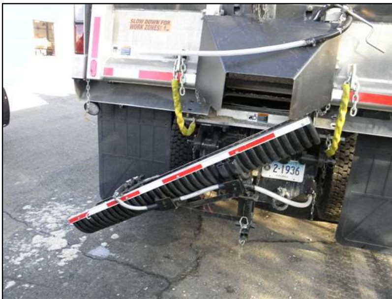
Figure 16: The Connecticut Rear Truck-Mounted Discharge Chute
